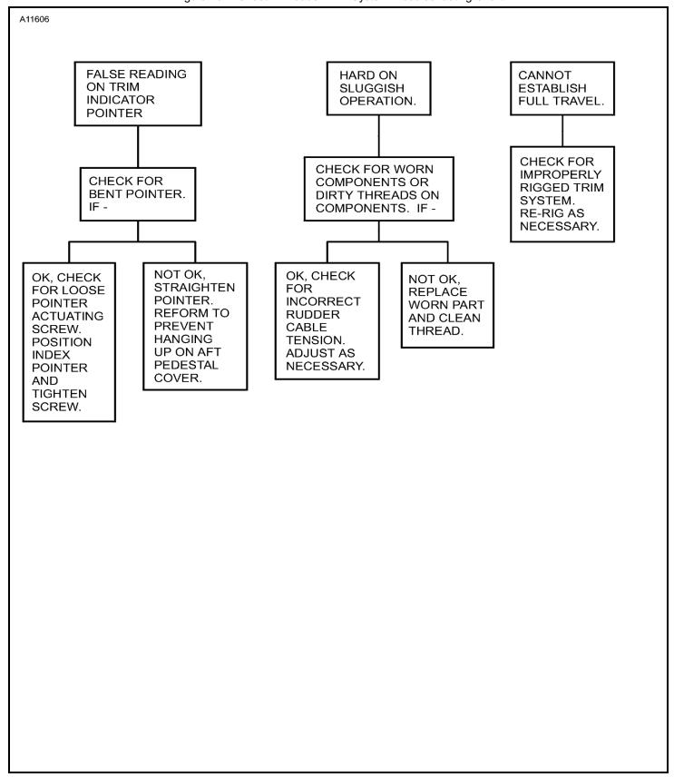
Figure 101: Sheet 1: Rudder Trim System Troubleshooting Chart
